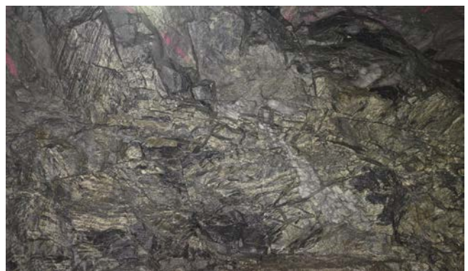
Figure 17: The highest grade areas of the mine are also high-sulphide. Take a look at how smashed up this rock is.
