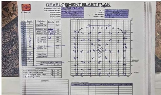
Figure 20: This is what a full face boring plan looks like. A lot of drilling and about a 1.5-2 hour cycle.
