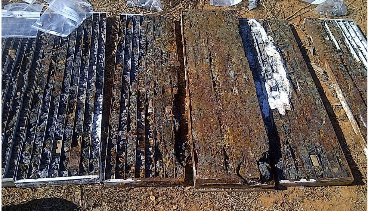
Figure 3: Heavily degraded drill core, during re-sampling
