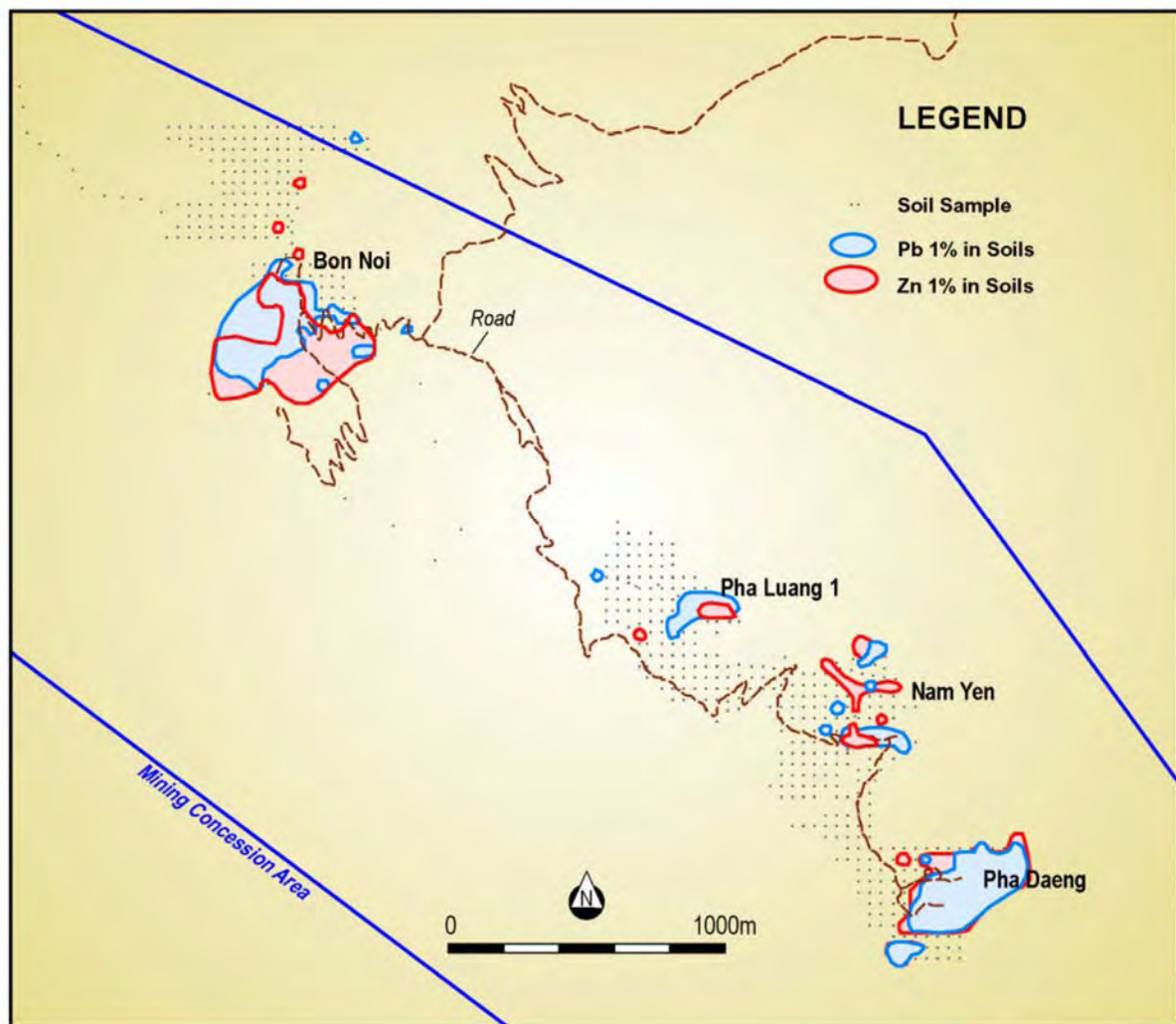
Figure 1: Pha Luang Project, showing overlapping soil anomalies at Bon Noi, Pha Luang 1, Nam Yen and Pha Daeng
