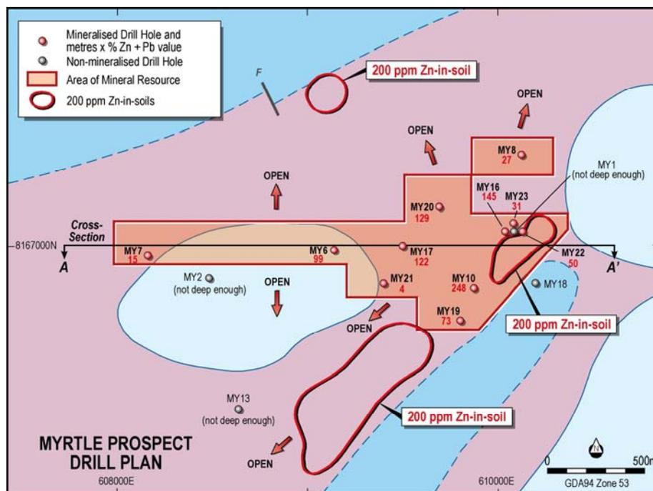
**Figure 1: Myrtle Prospect Drill Plan, showing interpreted geology, current resource blocks and soil anomalies**
